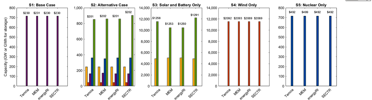
Fig. 1. (a) Initial and (b) final built generation capacities for each of the four models in each of the five cases. The units are in GW for natural gas, solar, wind, and nuclear capacities and GWh for battery storage. As can be seen in the y-axes, the built capacities for all models in case S3 and S4 are a factor of 10 greater than those for cases S1, S2, and S5. Also shown above each model are the corresponding total annual system costs (in billion dollars US) for each of the cases. Note that this is a 1-year simulation, so the total annual system cost equals the total system cost.
